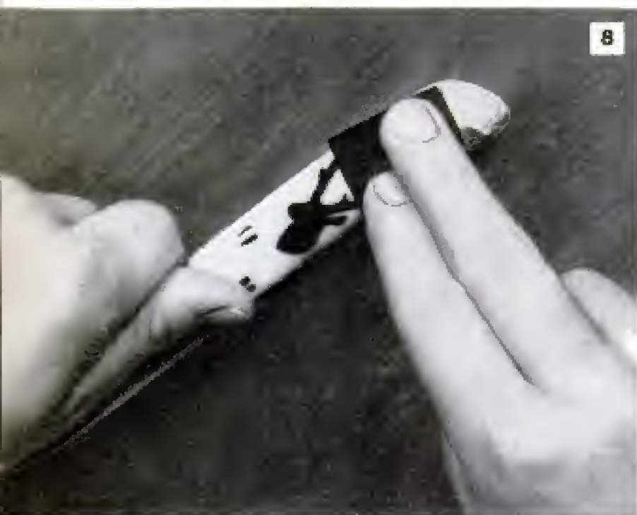
Roughly shaped handle is given a secondary sanding with 180-grit paper and then a final sanding with 320-grit paper, as above, both sandpapers being used wet. After sanding has resulted in desired shape, handle is given final polishing with cloth
